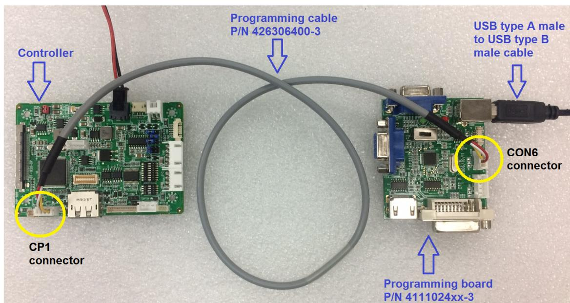
3. Insert 12V power source to PP2 connector and short JP6 / power on the DT-1920-DP .
