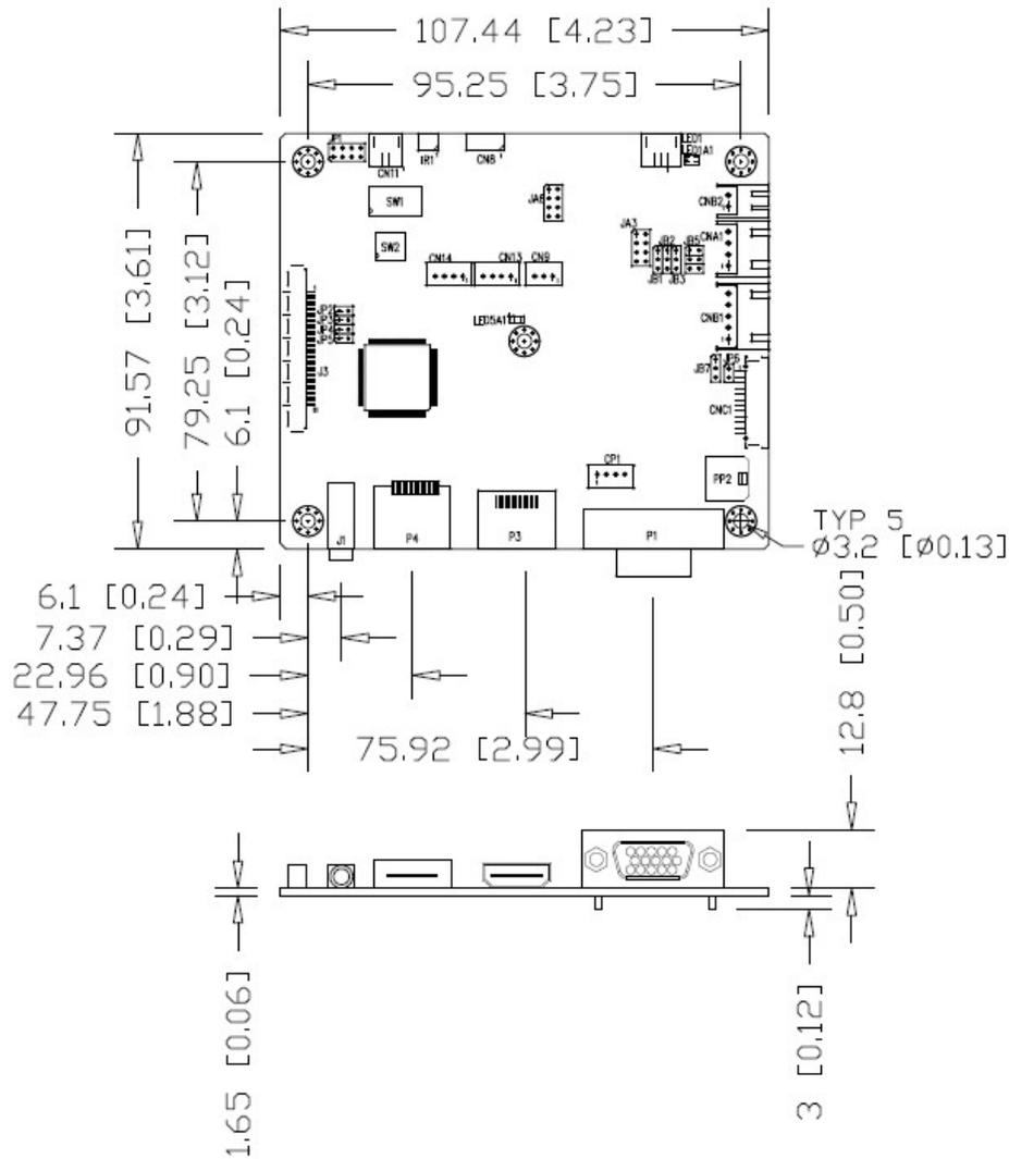
The maximum thickness of the controller is 17.45mm (measured from bottom of PCB to top of components, including any underside components & leads). We recommend clearances of:
