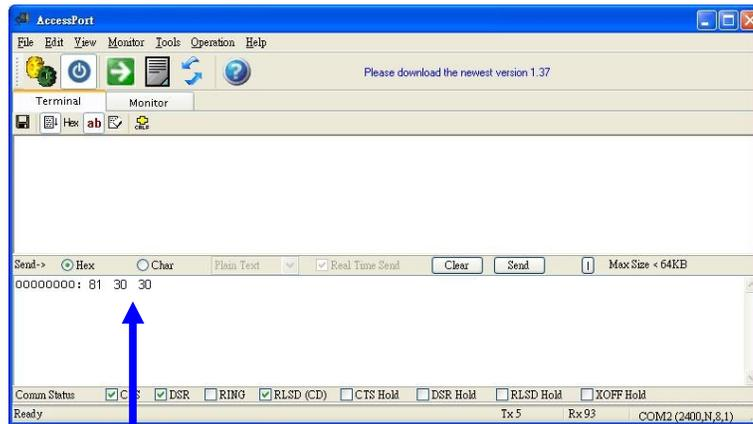
For example : Type "81 30 30" to adjust Brightness to min value. (0%)
