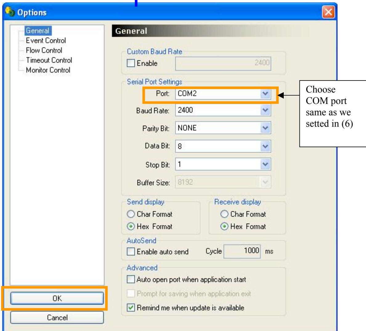
(8) Type RS-232 commands using serial communication program like “AccessPort” to control the controller function
