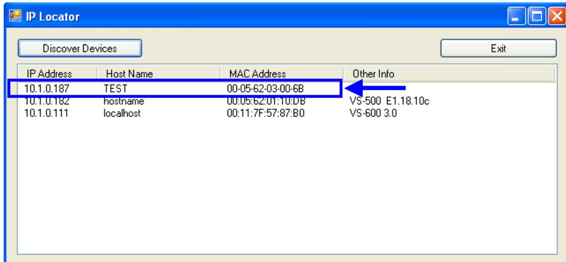
Browser Mode control uses a standard web browser to send commands to IP-60. To select browser mode, open the web browser after the IP-60 boot up, enter the corresponding IP address (e.g "10.1.0.187") in the address bar, then the following page will show up.
