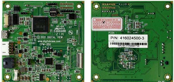
**EPM-050 Driver Board:** Designed specifically to support the E Ink 13.3" monochrome panels, the EPM-050 accepts bitmap images transferred over a USB connection. The images are then written to the panel immediately. The board has fast startup and ultra low standby power consumption of 0.01W (for 5V input).
